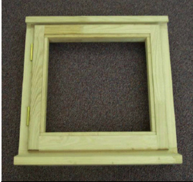
Green gluing: finger jointing and finished frame
